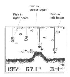
ID+ adds an additional piece of information to help the user locate fish. On selected fish symbols, the digital depth of the designated fish is drawn to help locate the fish vertically. This is especially helpful in setting bait depths or for downrigger operation.
